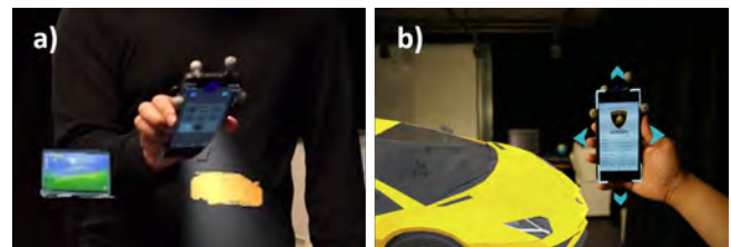
Figure 10. a) When the phone display is held away from the user, a flashlight is emitted, causing objects to be displayed in wireframe. b) When the phone intersects a 3D model, a detailed webpage about it is displayed on the phone.
