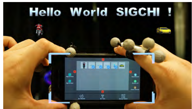
Figure 12. In Group Select mode, a swipe along the top of the phone performs a top alignment of the selected objects.
