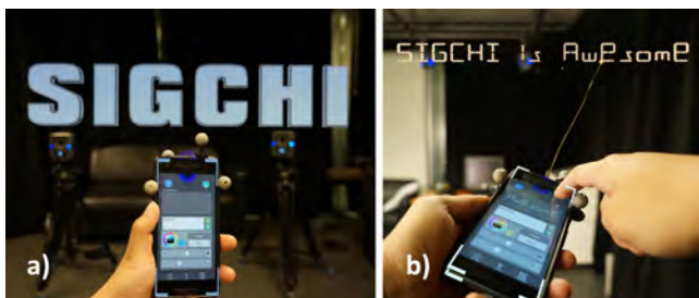
Figure 11. a) 3D text can be displayed in the 3D preview area. b) Text can be remotely edited on the phone.
