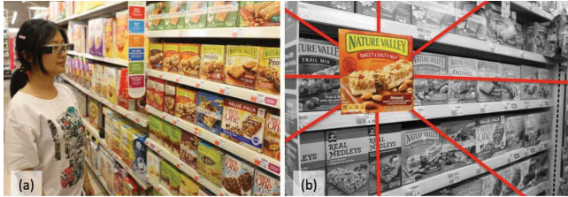
Figure 1. (a) An illustration of a low vision person using CueSee to facilitate a visual search task in a grocery store with augmented reality (AR) glasses. (b) The user sees visual cues, specifically designed for low vision, which direct her attention to the product.
