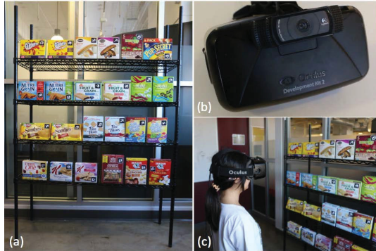
Figure 3. (a) A mock grocery store shelf with 24 products; (b) the video see-through HMD prototype; (c) a participant standing one meter away from the shelf conducting a product search task with CueSee.
