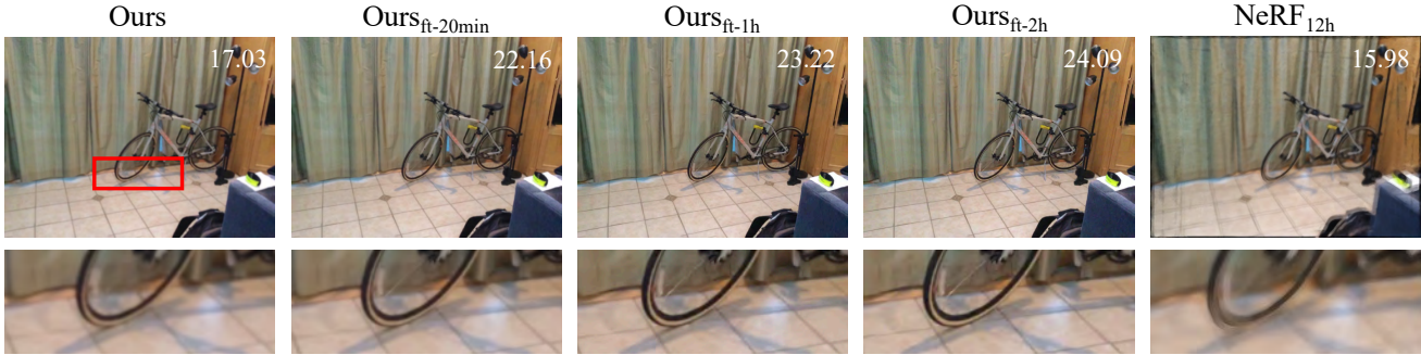
Figure 5. Effect of fine-tuning. We show the results with our model with different fine-tuning duration. The first column is our results without fine-tuning. Note that our direct inference result have outperformed NeRF and the results from fine-tuning contain significantly more details. PSNRs are shown at top right of each image.
