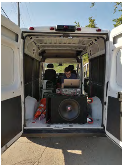
Figure 9: We loaded our signal generation apparatus into a van for mobility, which allowed us to test various distances in outdoor conditions.
