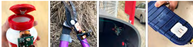
Figure 1. Four Sozu-augmented objects that use motion energy: pill bottle, garden pruner, mailbox, and slipper.
