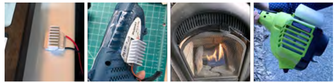
Figure 4. Sozu can be powered by hot surfaces, such as those found on stoves, hot glue guns, fireplaces, and gas tools.
