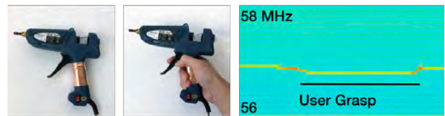
Figure 14. By including the user in the LC oscillator circuit via a conductive grip (copper tape), Sozu can detect user grasp, which manifests as a characteristic frequency shift.
