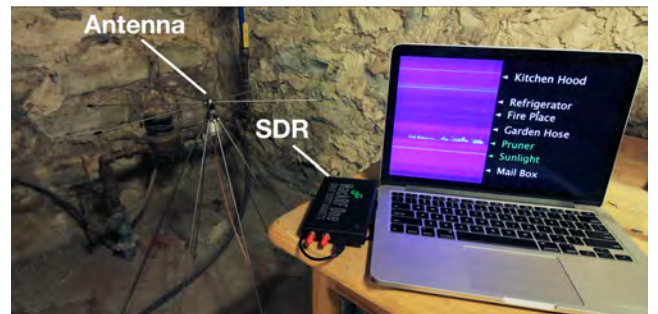
Figure 11. Sozu receiver setup deployed in a basement.
