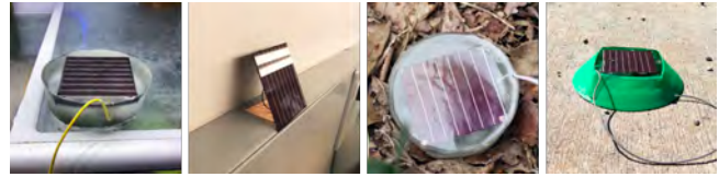
Figure 3. Sozu can also be powered by light energy: refrigerator door light, overhead work lights, and sunlight in a garden and parking lot.
