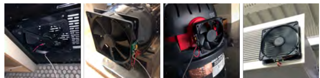
Figure 6. Sozu can be powered by gas flow from a kitchen hood, exhaust fan, ShopVac, and HVAC vent.
