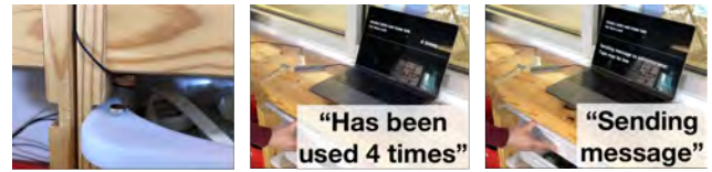
Figure 23. A Sozu-augmented storage bin can alert a shop manager to check on supplies after repeated access.
