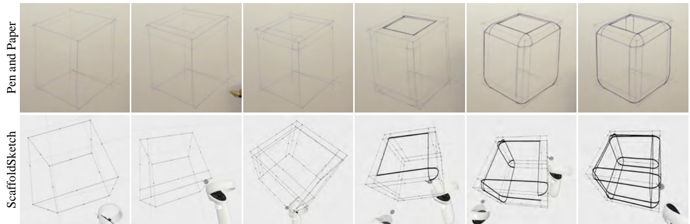
Figure 2: Top row: Frames from a time lapse pen-and-paper industrial design drawing (“Product Design Sketching with construction lines” © Chris Wilson). Designers first construct scaffolding and then draw the shape curves on top. Bottom row: The same two-stage design drawing process executed in 3D with ScaffoldSketch. The raw input and auto-corrected output for this example can be see in Figure 3.
