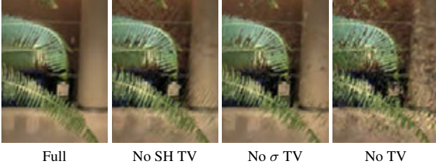
Figure 3. Ablation over TV regularization. Clear artifacts are visible in the forward-facing scenes without TV on both \sigma and SH coefficients, although PSNR does not always reflect this.
