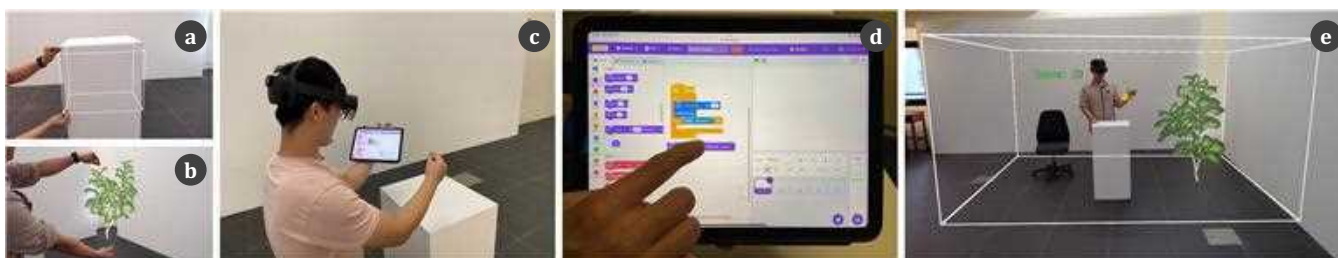
Figure 1: ProInterAR is an integrated visual programming platform for creating immersive AR interactions with a tablet and an AR-HMD device. (a)-(b) The AR creator specifies physical contents or creates virtual contents (i.e., a physical white box and a virtual tree) from the AR-HMD. (c)-(d) The creator programs the interactive behaviors of the created AR contents from a block-based visual programming interface in the tablet. (e) The creator executes, watches, and controls the programmed AR application in the AR scene. In this example, an AR game “pat and bounce” is created using ProInterAR : The player first uses his hands to pat a virtual ball to make it move in the AR space continuously. It will bounce when it collides with the AR contents (i.e., physical walls, ground, a physical box, a physical chair, and a virtual tree). If the player catches and pats the ball once by hand, the score will be added by one.
