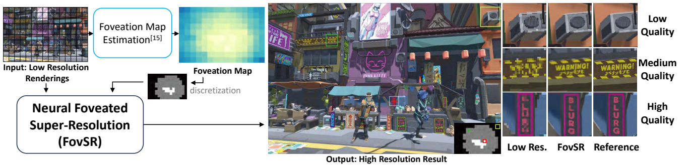
FIGURE 1 Overview of our foveated super-resolution method. We begin by generating low-resolution renderings using the native renderer. To determine the spatial visual quality required for each image patch, we estimate a luminance-contrast-aware foveation map 15 , considering factors such as eccentricity and content. After discretization, the foveation map categorizes image patches into different quality levels: low, medium, and high. Our neural foveated super-resolution method, referred to as FovSR, takes both the low-resolution rendering content and the discretized foveation map as input. FovSR uses this information to generate foveated high-resolution results that exhibit varying visual quality across distinct regions. For a more detailed examination of our results, zoomed-in crops are displayed on the right, offering a closer look at the output. The fovea is marked by a red cross.
