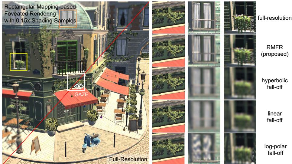
Figure 1: Left: Comparison of the proposed foveated rendering (upper-left) and the full-resolution rendering (lower-right). Right: As illustrated in the close-ups of the rendered images, compared with hyperbolic fall-off [9], linear fall-off [35], and log-polar fall-off with kernel functions [22], our method generally preserves sharper details on the peripheral regions with the same rendering budget.
