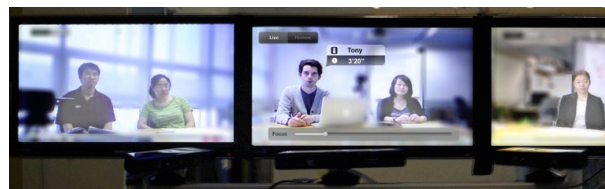
Figure 1. FocalSpace: active speaker in focus, inactive speakers dimmed 50%, and synthetic blur applied to background.
