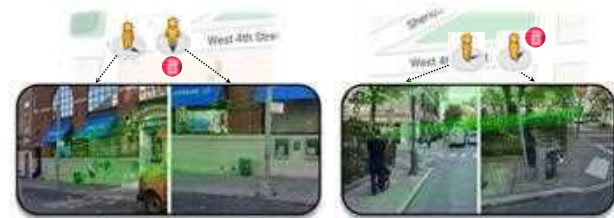
Figure 5. RX-399 avoids double-counting trash cans by identifying duplicates across different viewpoints using feature matching.
