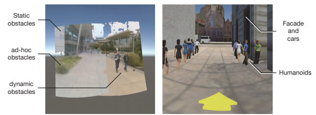
Figure 8. DreamWalker represents static obstacles through stationary virtual objects, such as buildings or cars. Ad-hoc and dynamic obstacles are represented through animated humanoid characters that walk towards the location of obstacles.
