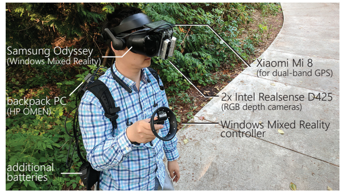
Figure 3. DreamWalker's mobile virtual reality system, including sensors, computing platform, and display device.
