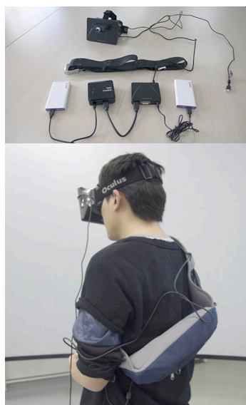
Figure 3. The wearable wireless transmitting system.
