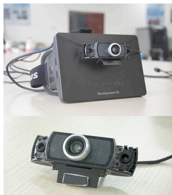
Figure 2. Modified the HMD with wide-angle lens camera.
