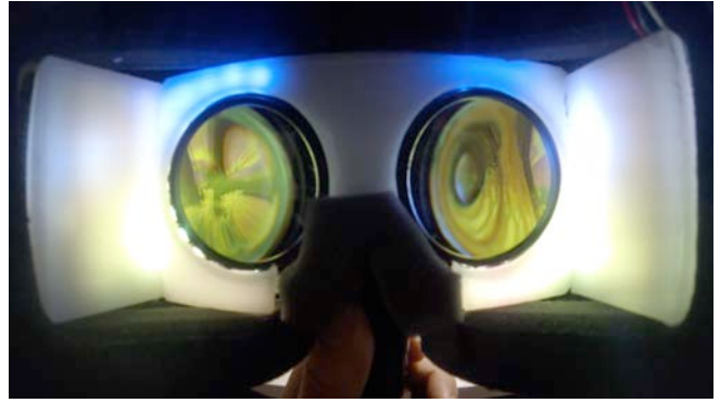
Figure 10. The forest scene used to introduce users to SparseLightVR. Left: the virtual scene as rendered for the Oculus Rift DK2. Right: scene as it appears inside the unit with SparseLightVR enabled.
