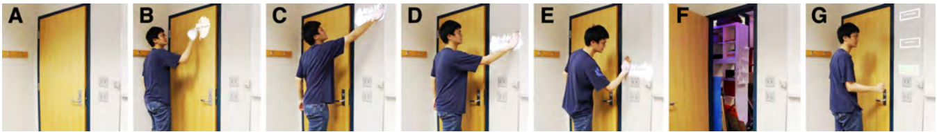
Figure 6. This sequence illustrates a user setting up a simple notification message application on an instrumented office door (A). First, a user “paints” a presence interactor on an office door (B), which can detect if the door is open or closed. The user then paints three contact interactors, labeled “in meeting”, “working” and “just knock”, onto the wall adjacent to the door (C, D and E). When the door is open, the application is invisible (F). When the door is closed, three buttons appear, which are user selectable (G).
