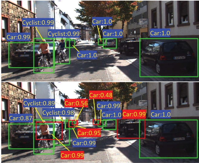
Figure 2: Comparison of object detection and classification, 2D (YOLOv4 on the top) vs. 3D (PV-RCNN at the bottom). PV-RCNN can detect more occluded and further away objects (with red labels) than YOLOv4.
