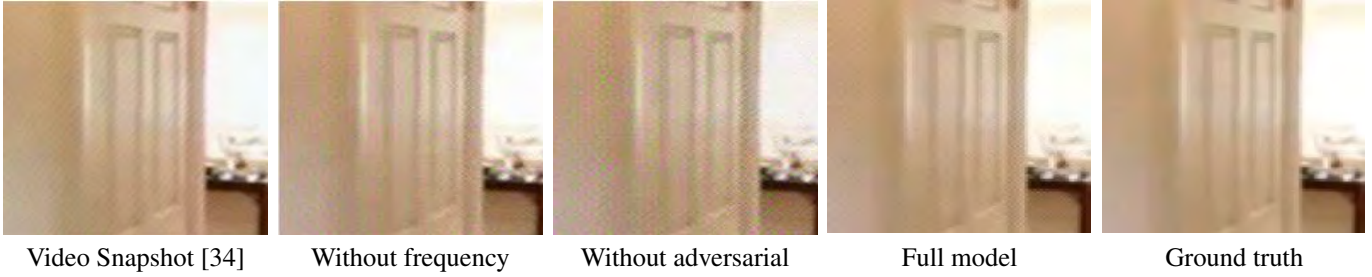
Figure 5. The comparison shows the effect of loss functions. Without the frequency loss and the adversarial loss, the embedding image has evident color strips and high-frequency artifacts. We recommend readers zoom in for the details.
