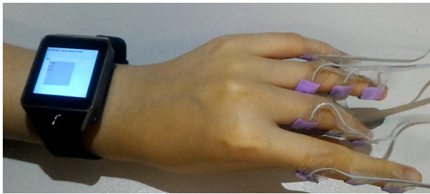
Figure 2: Experimental prototype of FingerT9 .
