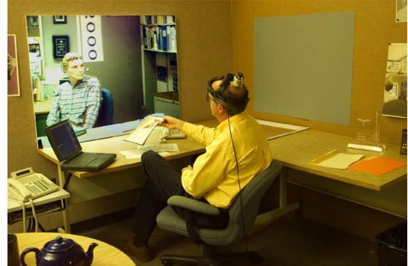
Figure 2: Portal to a distant office. Shown here in mono, the remote office scene is normally viewed in stereo by the head-tracked user.
