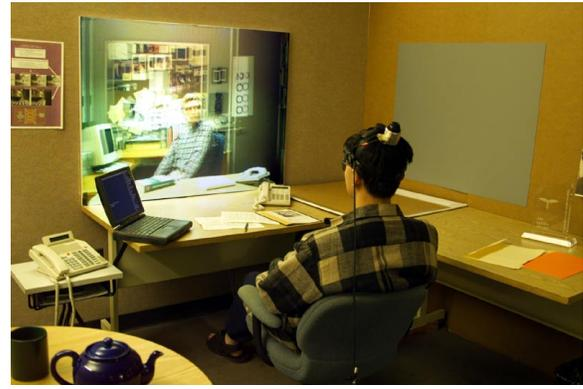
Figure 11: Working system with the tracker placed on the user's head and rendering in stereo mode.
