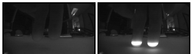
Figure 12. The Side Mouse camera image. Two fingers are hovering above the surface and are not illuminated (left). Once touching the surface, the IR beam is broken by the fingers and these become brightly illuminated (right).
