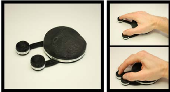
Figure 13. Arty Mouse is equipped with three high-resolution optical mouse sensors: one in the base, which rests under the user’s palm, and two under the articulated extensions that follow the movements of the index finger and thumb.
