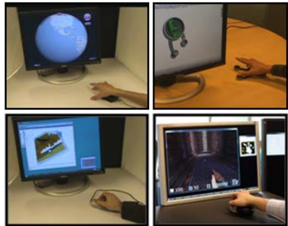
Figure 16. Applications running with our MT mice. Clockwise from top-left: manipulating Virtual Earth, 3D modeling in SolidWorks, controlling a first person shooter game and photo browsing using a desktop mockup.
