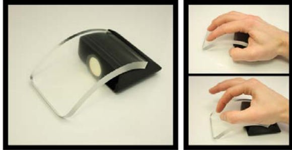
Figure 2. FTIR Mouse applies the principle of frustrated total internal reflection to illuminate a user’s fingers, and uses a camera to track multiple points of touch on its curved translucent surface.
