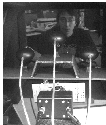
Figure 2. Back side of the Attentive Video Tunnel, with cover removed. Inside, 3 video cameras are mounted behind a half-silvered mirror. The eye tracker is visible below the cameras.
