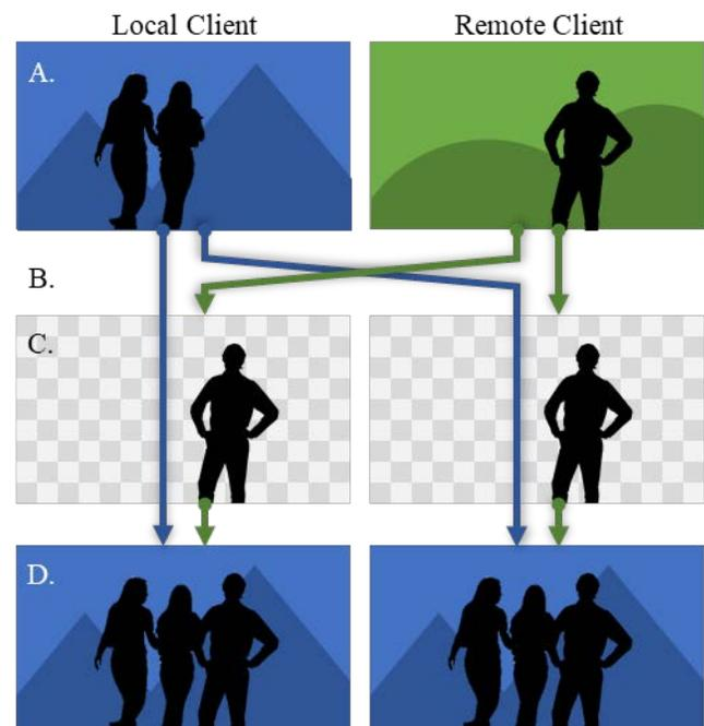
**Figure 1: Functional schematic of the prototype. Each client (A) captures the camera stream, (B) exchanges it with each other using WebRTC, (C) performs chroma key background removal on the remote client's video, and then (D) overlays it on the local client's video.**
