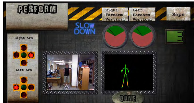
Figure 10: Performance interface. Information regarding static bones is displayed on traffic lights whilst the ranges of motion of dynamic bones are displayed on dials. The user can see the video recording of the demonstration and his own skeleton as tracked by the Kinect with each bone in a different colour depending on its score. The interface also displays the repetition count and warnings when the speed is too fast or too slow.
