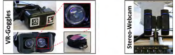
Figure 2: Hardware setups: a source actor experiences VR wearing an Oculus DK2 headset (left). We track the source actor using a commodity RGB-D sensor (front-facing), and augment the HMD with ArUco markers, as well as an IR webcam in the inside (mounted with Add-on Cups 2 ). The target actor footage is captured with a lightweight stereo rig, which is composed of two webcams (right).
