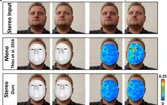
Figure 11: Stereo alignment: we compare the photometric alignment accuracy of our approach to Face2Face [2016]. Face2Face only obtains a good fit to the image captured by the left camera (average error of 0.011), but the re-projection to the right camera suffers from strong misalignments (average error of 0.019). In contrast, our stereo tracking method obtains consistently low errors for both views (average error of 0.011 left and 0.012 right).
