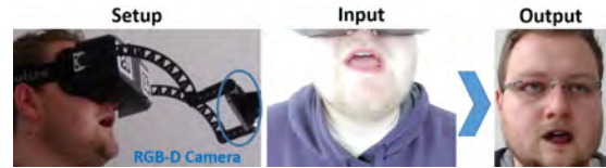
Figure 16: A setup with a rigidly mounted RGB-D camera (Intel Realsense F200) allows for cross-projection of the mouth independently of the head rotation.
