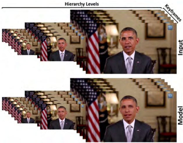
Figure 10: Non-rigid model-based bundling hierarchy: the top row shows the hierarchy of the input video and the second row the overlaid face model.
