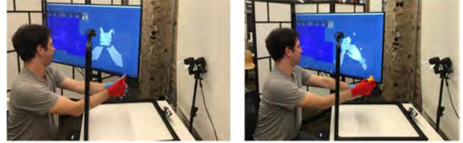
Fig. 8. Our three camera rig captures depth data from three views at 180 fps. We use calibrated RGB cameras to perform segmentation of the two hands, each contained in a different glove from both each other and other objects.
