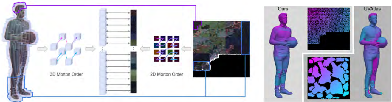
Figure 4: Texture packing – (left) 3D blocks and 2D patches are ordered and matched by their Morton codes respectively. This process unwraps the 3D volume to the texture atlas. (right) The UVAtlas [71] only ensures local spatial coherence within each chart, whilst our method encourages global spatial coherence. Refer to the supplementary video for a comparison on temporal coherence.
