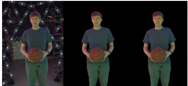
Figure 9: Texture / Qualitative – A frame taken from the comparison sequences in the supplementary video : (left) raw rgb image from camera; (mid) rendered with UVAtlas [71]; (right) rendered with our texture atlas. there is no visible difference in quality.
