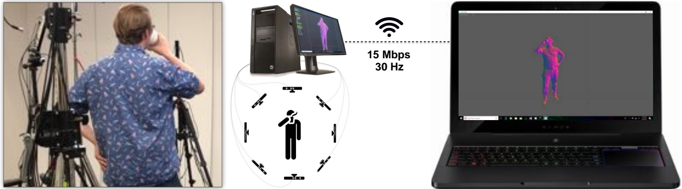
Fig. 1. We acquire a performance via a rig consisting of 8× RGBD cameras in a panoptic configuration. The 4D geometry is reconstructed via a state-of-the-art non-rigid fusion algorithm, and then compressed in real-time by our algorithm. The compressed data is streamed over a medium bandwidth connection ( \approx 20 Mbps), and decoded in real-time on consumer-level devices (Razer Blade Pro w/ GTX 1080m graphic card). Our system opens the door towards real-time telepresence for Virtual and Augmented Reality – see the accompanying video.
