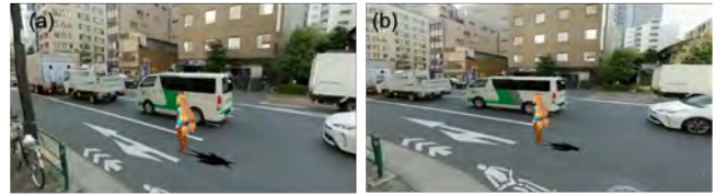
Figure 2: The effect of the projection: (a) In a spherical projection, the avatar seems to float. (b) In the proposed elliptical projection, the avatar appears as a part of the scene.
