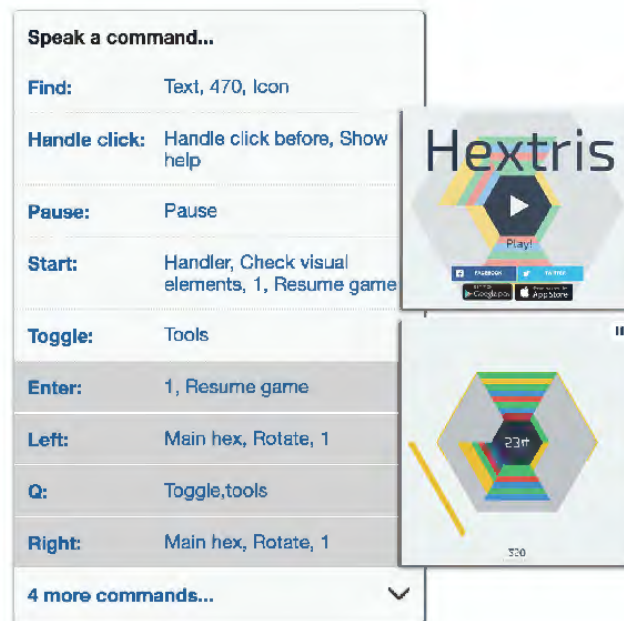
Figure 6.2: The Hextris web game (hextris.io) shown with a list of speech commands created by Genie. Speaking the bolded text label for each command triggers the corresponding actions.
