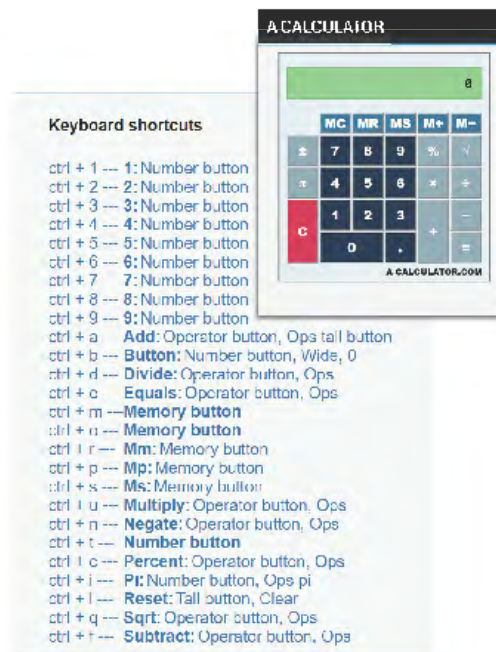
Figure 6.6: A calculator interface with incomplete keyboard support (a-calculator.com), enhanced to provide a keyboard shortcut for each command, as enabled by Genie’s analyses.
