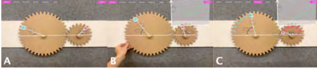
Figure 17. Explanation of gear ratios: The teacher explains the angular motion of different sized gears.
