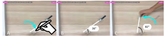
Figure 8. Angle: The user can draw a path between lines (A), and the system parameterizes it as an angle (B). The angle can be dynamic if the line is bound to the object (C).
