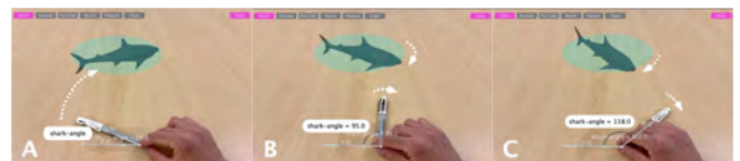
Figure 21. By mapping the defined variable to an angle property of the virtual object, the user can quickly craft an improvised tangible dial to rotate the virtual object.
