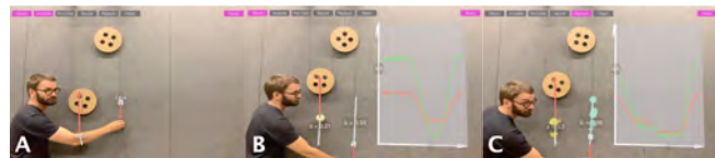
Figure 15. Pulley system experiment: The user measures the distance of a hand movement and a load, and visualizes it with a graph (green: hand movement, orange: the load).
