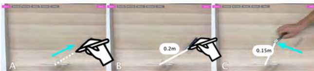
Figure 7. Line segments: Sketch a line on the screen (A). If the line is attached to the tracked object (B), it becomes bound to the object (C).
