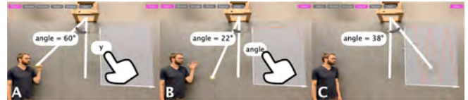
Figure 12. Plotting a graph: By binding an axis label with an existing dynamic variable (A-B), the user can plot a real-time graph of the parameter (C).
