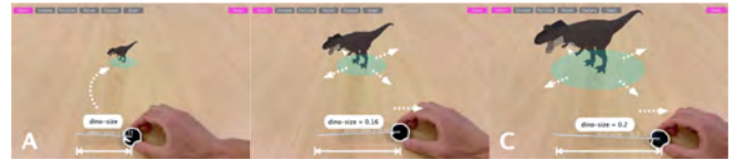
Figure 20. In-situ creation of a tangible UI slider: The user binds the object distance to the scale of the virtual 3D model, so that the model size changes as the object moves.
