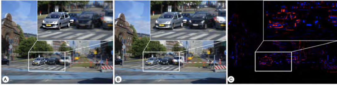
Figure 2: Differences in saliency modulation methods not considering additive only properties of OSTHMDs exemplified by our implementation of the algorithm by Mendez et al. [38] (insets for details): (A) Full colour control allows increasing the saliency of some image elements (e.g., silver car) while decreasing the saliency of other elements (e.g., black car). (B) Modulation using only the additive components fails to demonstrate the full saliency modulation. (C) Visualisation of required additive (red) and subtractive (blue) modulation necessary to highlight the silver car showing the majority of image areas are modulated by subtractions that are not possible in OSTHMDs.
