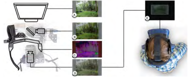
Figure 6: Study apparatus: (A) Scene displayed on a screen representing the real environment is captured by the scene camera (B). The computed saliency modulation (C) is then displayed on the AR glasses. The combined view (D) captured by the user-perspective camera (representing the human eye) is finally displayed in the virtual environment (E).
