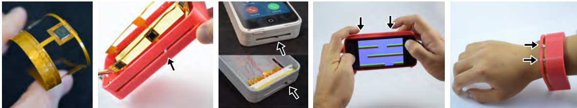
Figure 1: Reconfigurable tactile elements (shown in arrows) for interaction on a mobile device. Left to right: a flexible PCB utilizing micro-coils for magnetic actuation of tactile elements, a mobile prototype using the PCB micro-coil technique, a mobile prototype using low-power switchable permanent magnet actuation, a game played using reconfigurable tactile controls, a wearable band with tactile elements for display and interaction.
