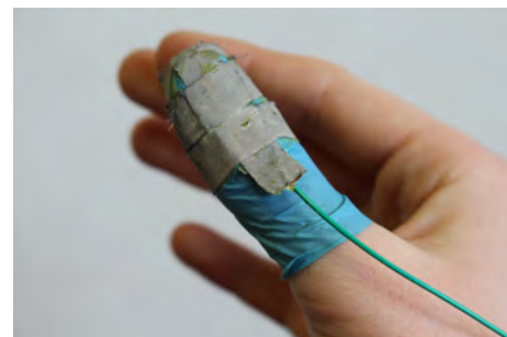
Figure 7. Automatic ground-truth annotation of thumb-to-finger touch using a capacitive finger glove, built out of nitrile rubber with conductive fabric affixed around the tip of the finger.
