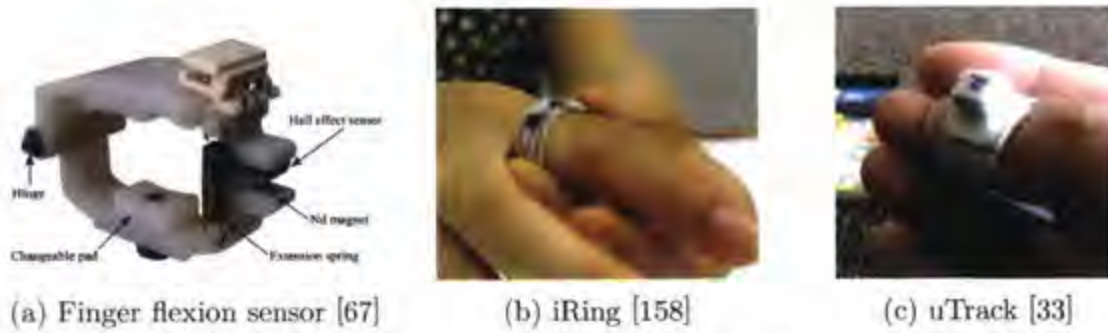
Figure 2-6: Input modalities in finger-worn devices. (a) a sensor for the flexion of finger tendons, (b) an IR reflectance sensor for different parts of the finger’s skin, (c) a magnetic sensor. Images courtesy of authors.
