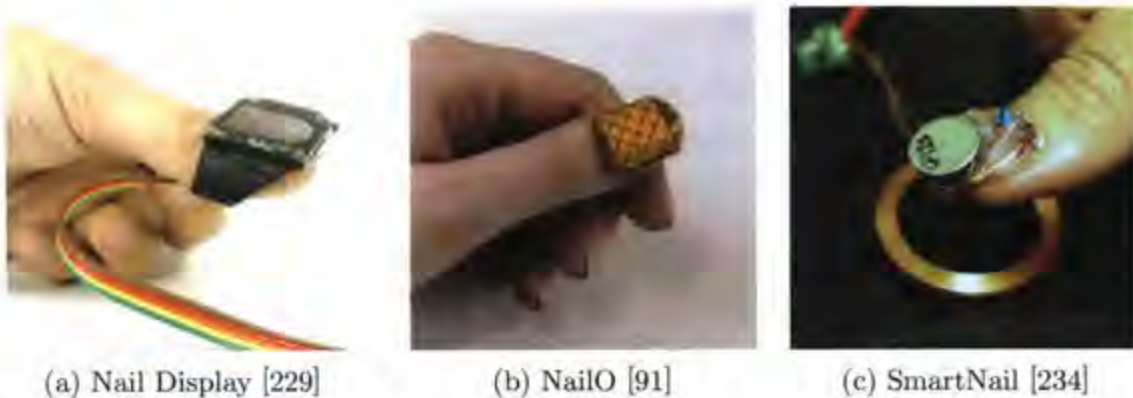
Figure 2-5: Finger-nail augmenting devices: (a) a miniature display added to the thumb, (b) a touch-sensitive pad for 2D cursor control, and (c) a radio controlled vibration motor.
