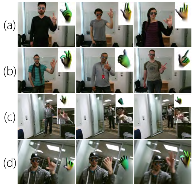
Figure 6: Our system (a,b) can track a wide variety of users and hand shapes, (c) can track at both close and far ranges, and (d) is robust to both scene and user motion.
