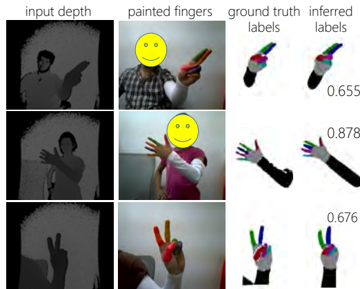
Figure 11: Examples from our FINGERPAINT dataset. For each row, we see the input depth image, the calibrated RGB image in which the painted fingers can be seen, the resulting ground truth labeling of the depth image, and the inferred labels that our tracker produces. (Numbers shown are classification accuracies).
