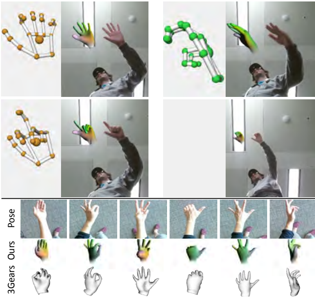
Figure 7: Top half: qualitative comparison of Leap Motion (left panels) with our method (right panels). Bottom half: qualitative comparison of 3Gears (bottom row) with our system (middle row). See text and video.
