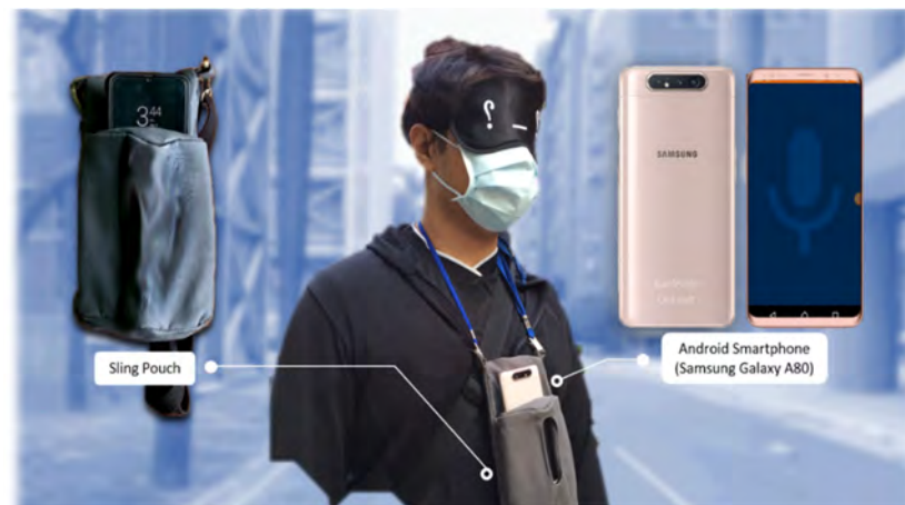
Figure 2. Proposed wearable mobility assistive system by using Android smartphone (right) and sling pouch (left).
