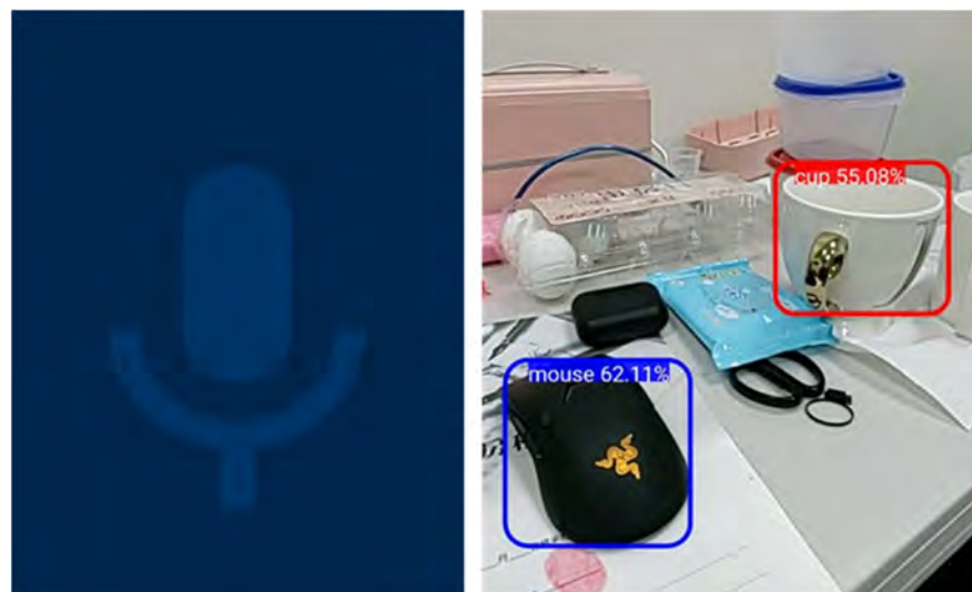
Figure 6. Object detection module with the voice command interface (left) and sample object detection result (right).
