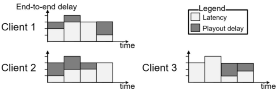
Fig. 32 AES. The latency estimation from the loss and delay is used to calculate the necessary end-to-end delay to equilibrate the timings of all clients
