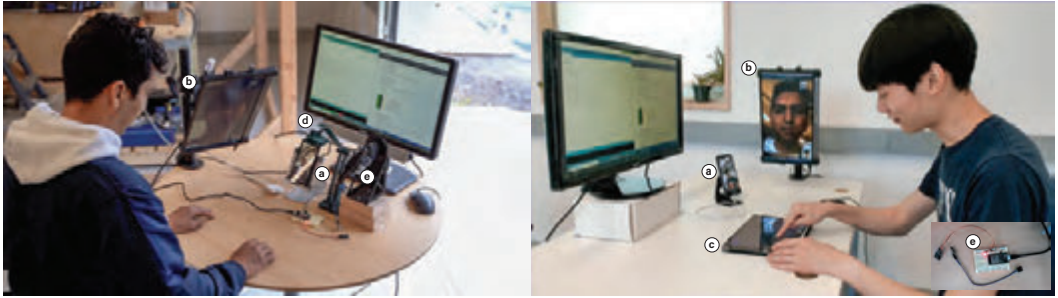
Fig. 1. A typical RemoteCoDe debugging session. At both sites, a TrueDepth camera (a) tracks the local user's head, and an embodied proxy (b) renders the remote user's locus of attention. The user can observe and point to the circuit using a tablet (c) connected to a document camera (d) and an actuated laser pointer (e).
