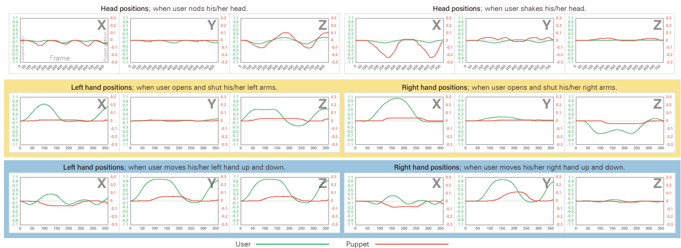
Figure 7. Result from captured 3-axes position of the puppet and user with 4 kinds of movements. Note that the maximum values of the vertical lines differ between the green line (user) and red line (puppet).
