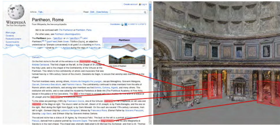
Figure 1: Given a reference text describing a specific site, for example the Wikipedia article above for the Pantheon, we automatically create a labeled 3D reconstruction, with objects in the model linked to where they are mentioned in the text. The user interface enables coordinated browsing of the text with the visualization (see video).
