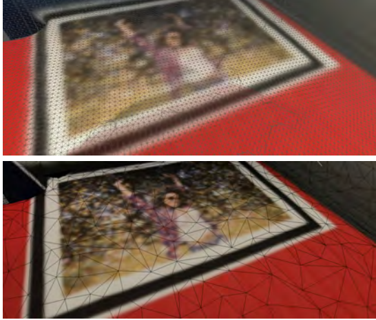
Figure 6. Different color representations ( top ) color per vertex; ( bottom ) texture per face; in the latter case, the mesh is 25 times lighter while the quality of texture is independently higher.
