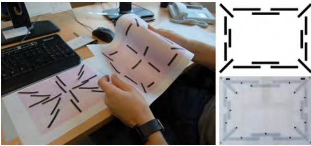
Figure 4: Paper prototyping to evaluate designs further (left). Our final layout (top right) and final printed clear surface (bottom right) is an optimal trade-off between limited amount of sensors and strong deformation sensing capabilities.
