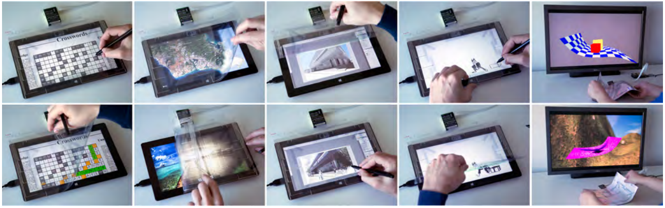
Figure 10: Example applications created using our sensor. A transparent tablet cover example, which acts as a magic lens revealing hidden metadata, applying rendering effects in photoshop, supporting window management, and allowing paper-like digital animation. Far right: using the foil as a high DoF 3D controller.
