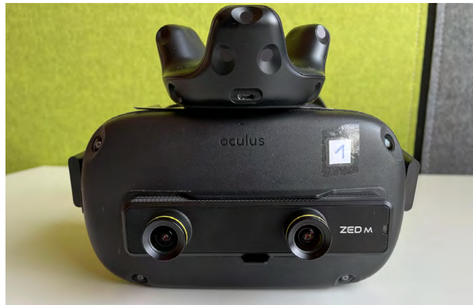
Figure 4. Oculus Quest with an attached Vive Tracker and ZED-Mini camera used in the evaluation.
