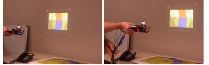
Figure 7: Quasi-stabilized projection translates with the user but maintains an upright rectangle with correct aspect ratio.
