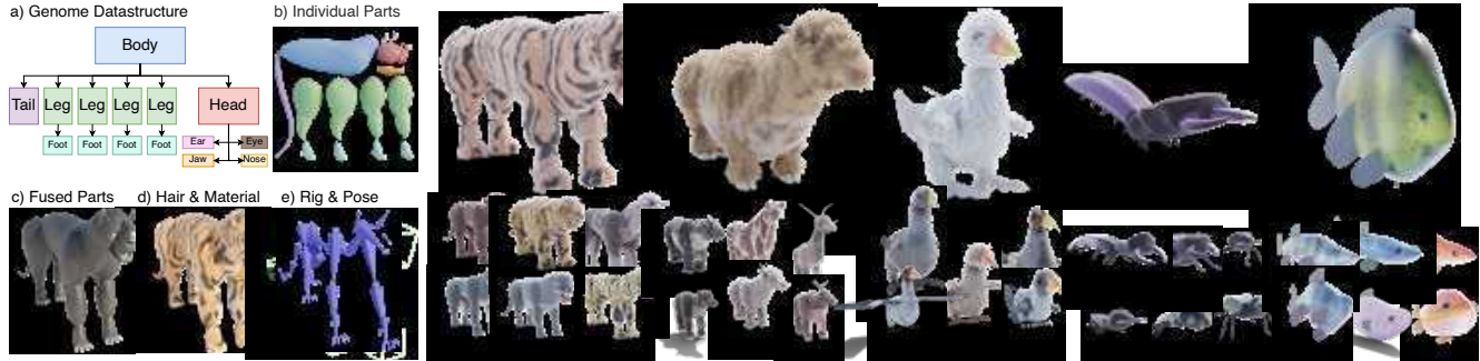
Figure 12. Creature Generation. Our system automatically generates genomes (a), parts (b), assembly (c), materials (d) and animation rigs (e). On the right, we show random, non cherry-picked samples from our Carnivore , Herbivore , Bird , Beetle , and Fish generators.
