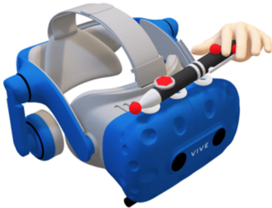
Figure 8: Illustration of a pen with hexagonal touchpad/button magnetically snapped to the top of a headset for convenient pickup and storage.
