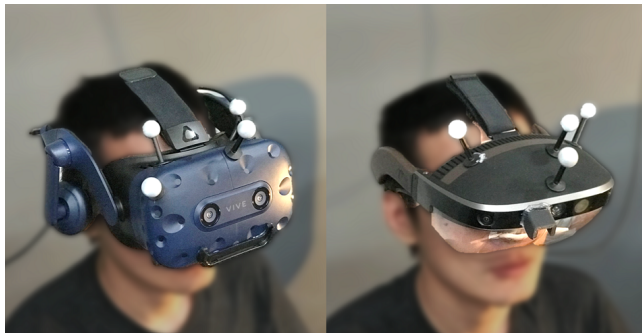
Figure 3: Left: HTC Vive Pro with 4 reflective markers. Right: Meta 2 with 4 reflective markers.
