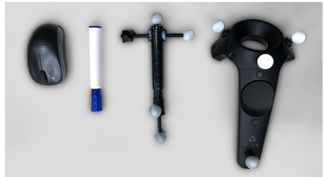
Figure 4: From left to right: (a) Mouse, (b) Standard whiteboard pen, (c) Wrapped whiteboard pen with 4 reflective markers, and (d) Vive controller with 4 reflective markers.
