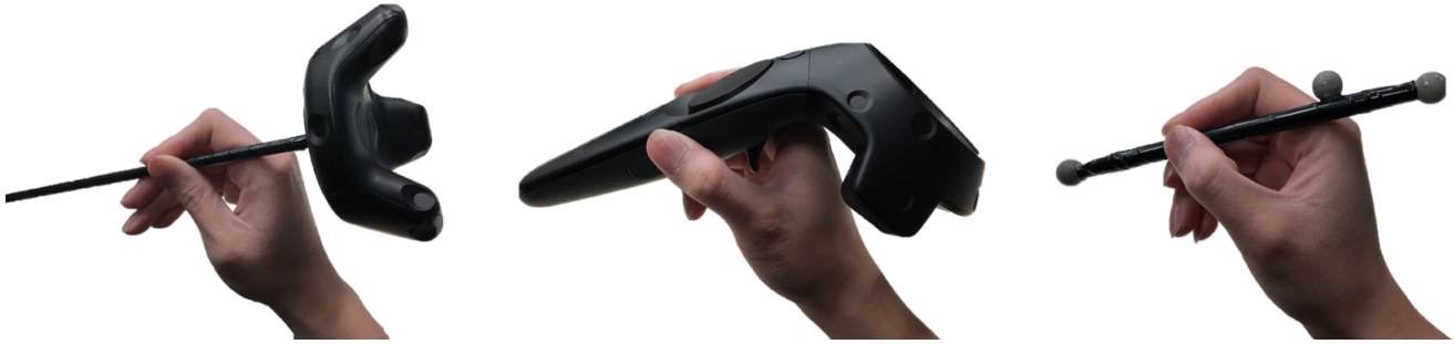
Figure 2: Prototypes explored during the design process. Left: Pen tracked by Vive Tracker. Middle: HTC Vive controller used as a pen. Right: Ballpoint pen device. All these did not perform well in our pilot studies.
