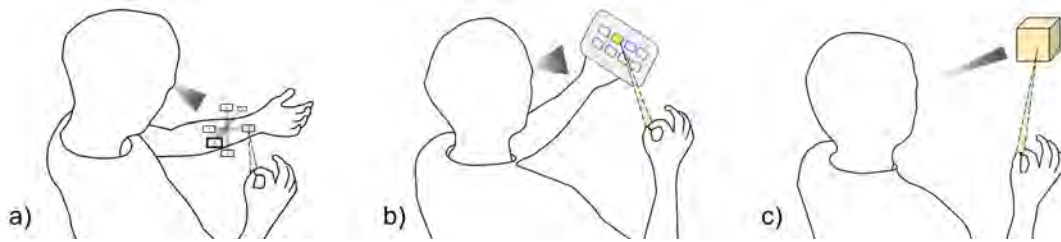
Figure 4: UI system: users can switch between interaction with the VEIA menu (a), hand menu (b), and objects at a distance (c).
