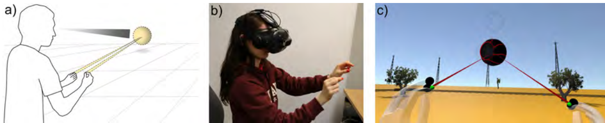
Figure 1: Gaze + Pinch interactions unify a user's eye gaze and hand input: look at the target, and manipulate it (a). Virtual reality users can utilise free hand direct manipulation (b) to virtual objects at a distance in intuitive and fluid ways (c).
