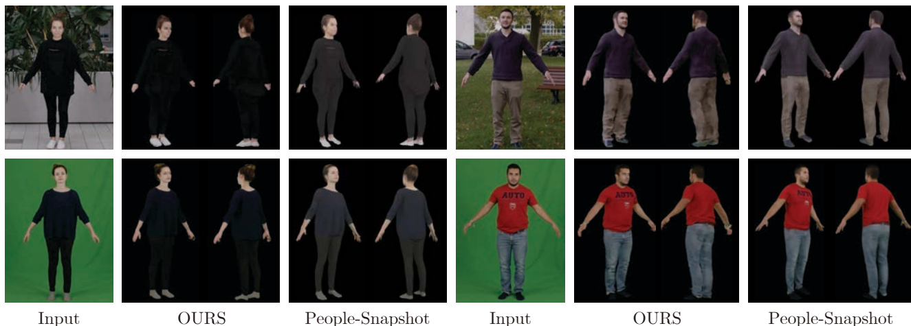
Figure 6: Novel view synthesis on monocular videos. Our method renders more appearance details than People-Snapshot [2], such as the blouse of the first person and the pants of the second person. Zoom in for details.
